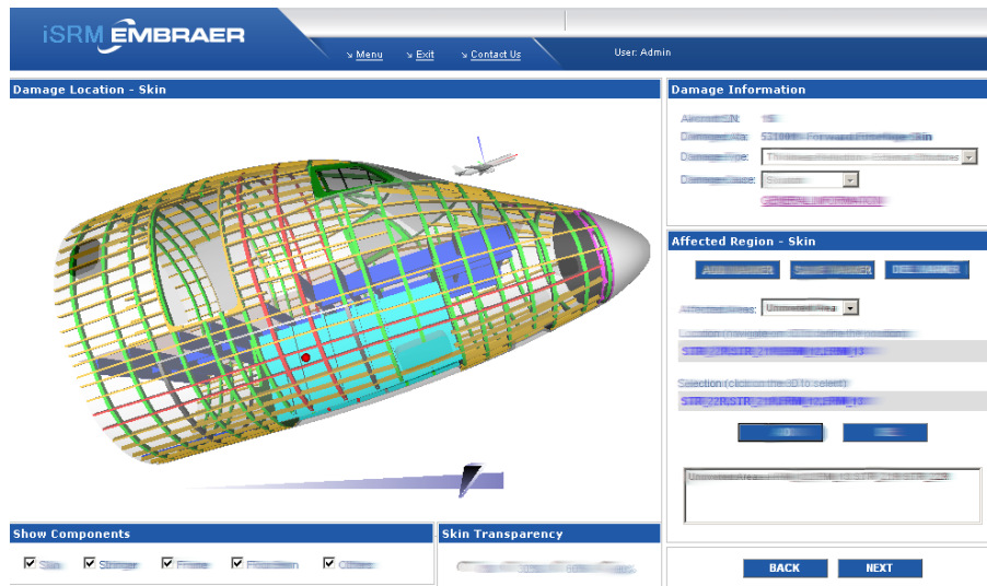
Figure 2. Graphic interface for damage characterization.
