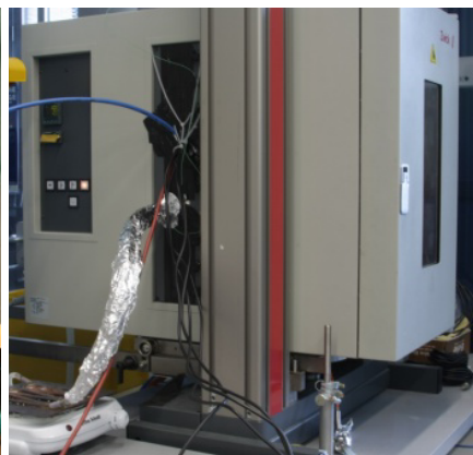
Figure 8. Setup with heating chamber.
