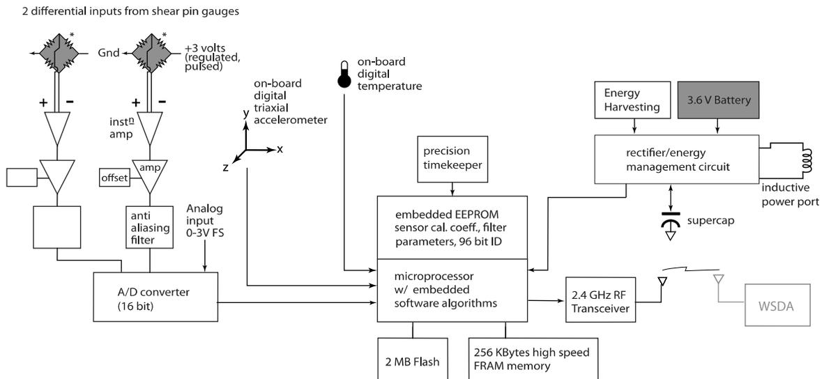
Figure 3. Block diagram of WISP microelectronics (SG-Link-MIL) and base station (WSDA-MIL). Two full bridge channels were monitored from each side of the V-22 nose gear trunnion to provide four channels of shear pin loads data.
