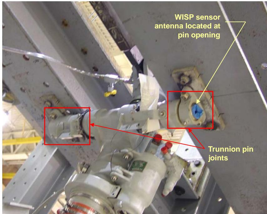
Figure 5. WISP trunnion pin installed in V-22 full scale testing rig.
