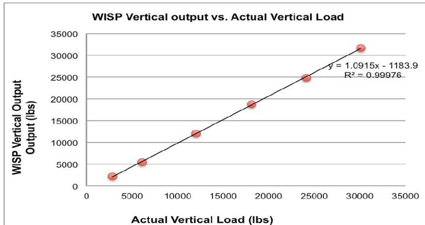
Figure 6. WISP output load using laboratory calibration data as a function of actual vertical loads applied to the V-22 nose landing gear in Boeing’s full-scale test rig.
