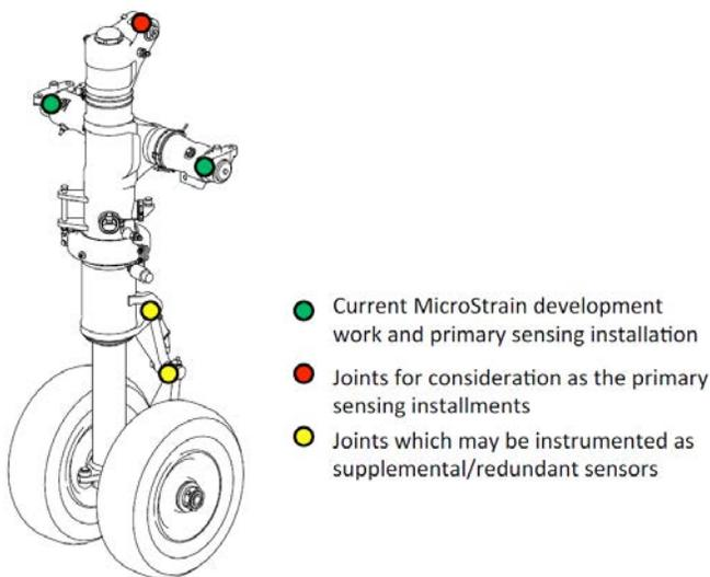
*Figure 2. Representative drawing of V-22 nose gear with locations for time-synchronized wireless integrated shear pins (WISPs). Primary measurement points are shown in green and red, and secondary (redundant) points are in yellow. In the present work, the green locations were instrumented.*
