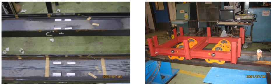
Figure 2. Deployment of strain gauges and bogie for vehicle simulation.
