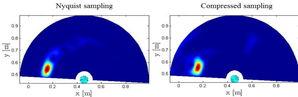
Figure 7. Imaging of  $170^\circ$  acoustic source.
