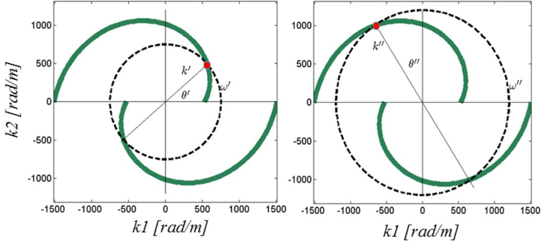
Figure 1. Schematic intersection of a wavenumber spiral distribution (green solid line) with dispersion circumferences at two different frequencies ( $\omega'$  and  $\omega''$ ).
