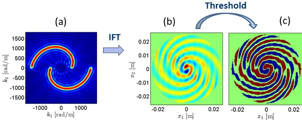
Figure 2. FSAT electrode design procedure: from the load distribution in the wavenumber domain (a) to the one in spatial domain (b) through IFT, then the 3-level quantization produces the electrodes' mask (c).
