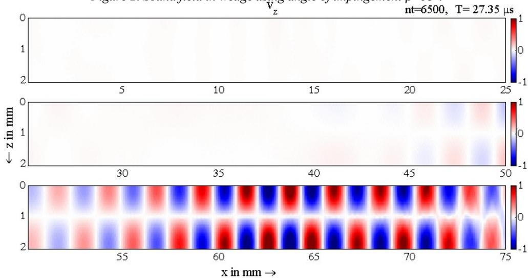
Figure 3. Lamb wave propagation of the  $S_0$  mode in a 2 mm steel plate (first 75 mm is shown here) at a frequency  $f=1.5$  MHz with a phased array transducer using angle of impingement  $\beta=53^\circ$ .
