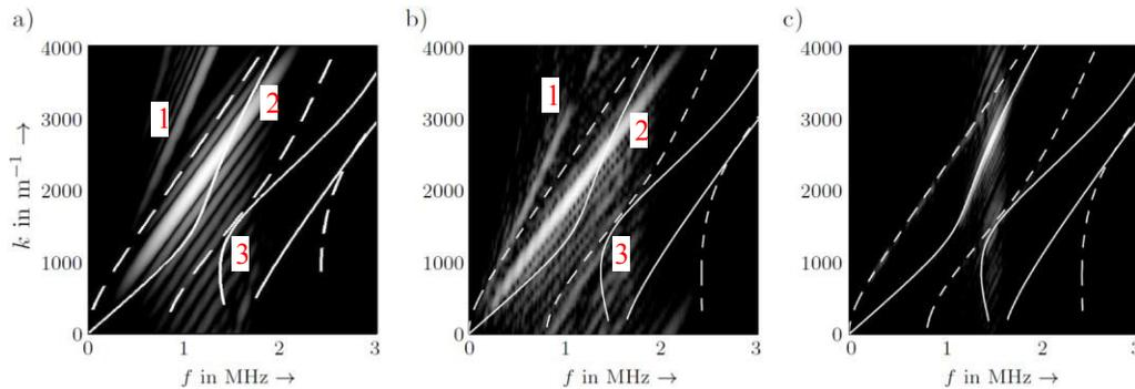
Figure 4. Excitation of  $S_0$  mode for angle of Impingement  $\beta = 52^\circ$ : a) simulated and b) measured spectra at the wedge base; c) excited modes in the plate. Scaling from -30 dB (deepest black) to 0 dB (brightest white). Marked: theoretical dispersion curves for the first three symmetric (-) and anti-symmetric (- -) modes.
