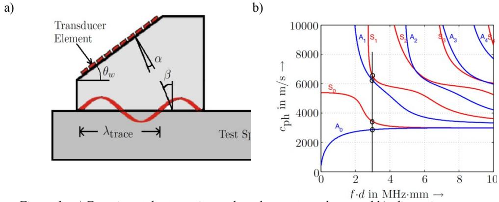
Figure 1. a) Experimental setup using a phased array transducer and b) dispersion diagram for a steel plate with thickness  $d=2$  mm.
