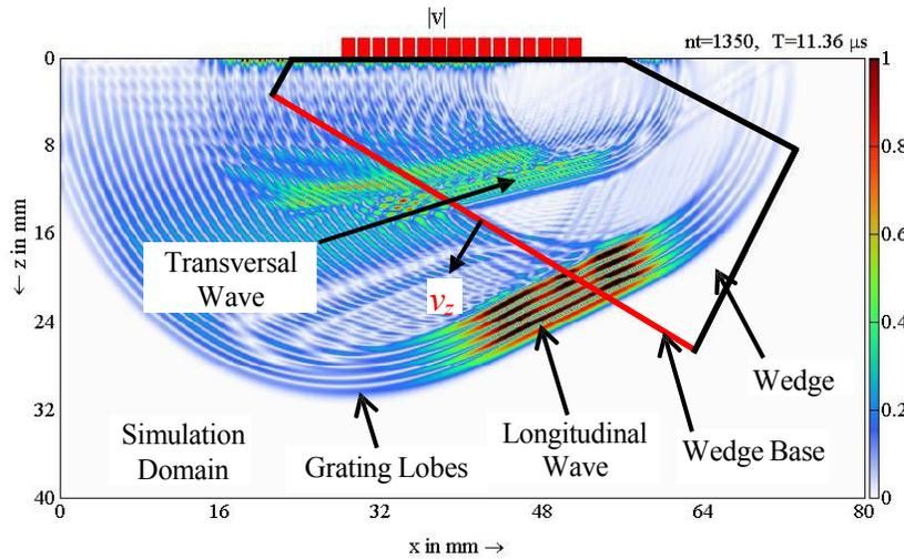
Figure 2. Sound field in wedge using angle of impingement  $\beta=53^\circ$ .
