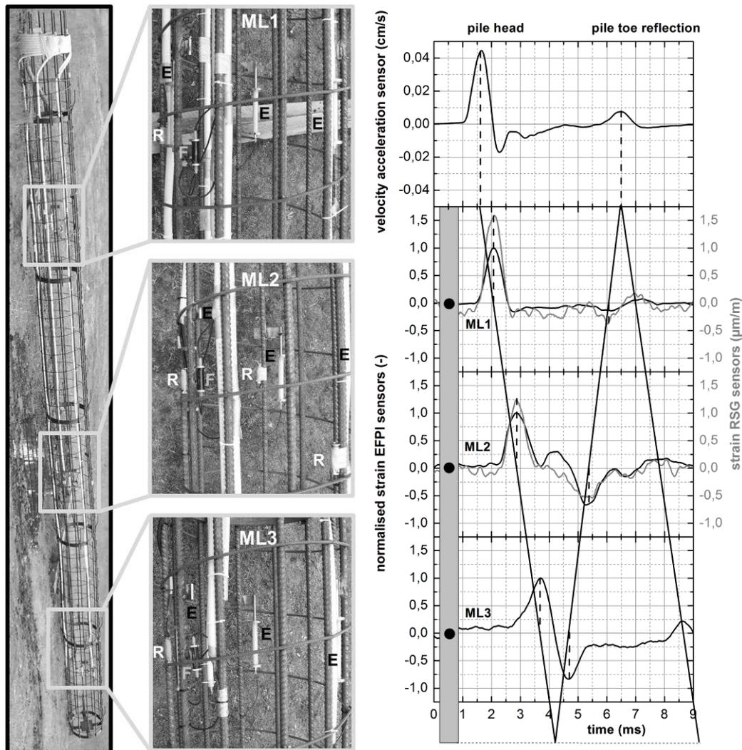
Figure 6. Left: Reinforcement cage with installed EFPI sensors (E), FBG sensors (F) and RSG sensors (R), right: wave propagation after low-strain impact.
