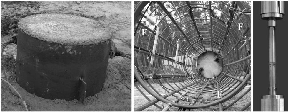
*Figure 7. Left: Pile equipped with fibre optic sensors, middle: reinforcement cage with two EFPI sensors (E) and one FBG sensor (F) at each measurement level, right: FBG sensor with temperature compensation.*
