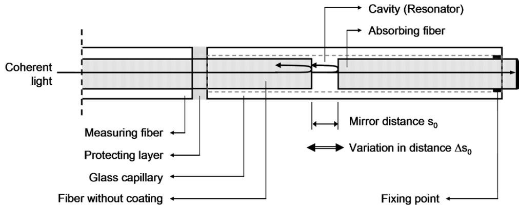
Figure 1. Flexible EFPI sensor.
