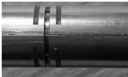
Figure 2. Flexure with applied flexible EFPI sensor.
