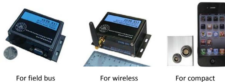
Figure 4. A series of PZT sensor network based digital impact monitors.
