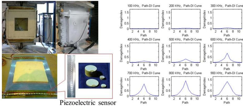
Figure 10. Photograph of the active SHM system for disbond detection in the thermal insulation system, and the damage index curves with different frequency.
