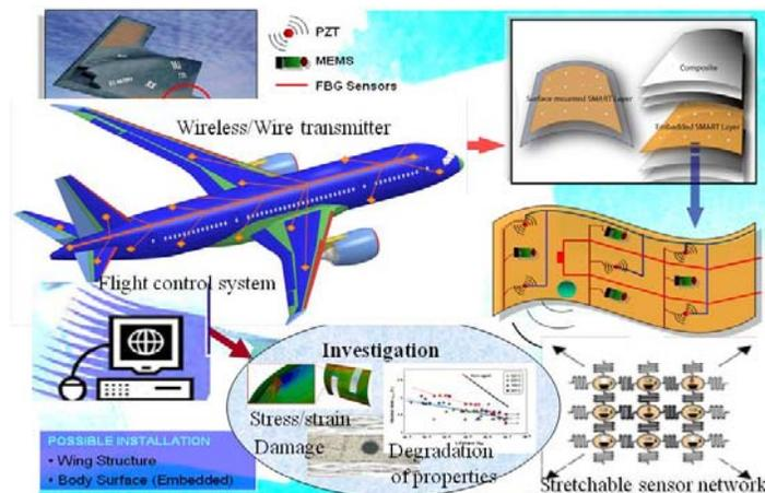
Figure 7. Concept of distributed multi-modal sensor network.
