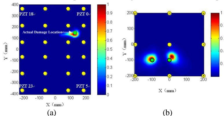
Figure 1. The imaging results for (a) single damage, (b) dual damages on composite structures.
