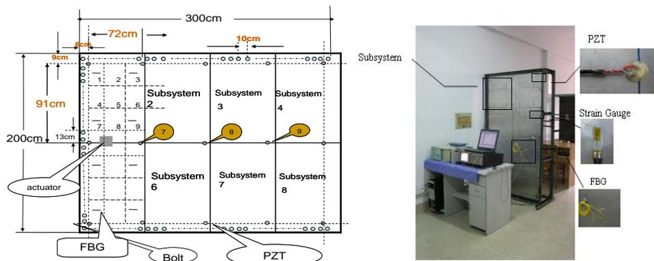
Figure 6. The multi-agent based structural health monitoring evaluation system.
