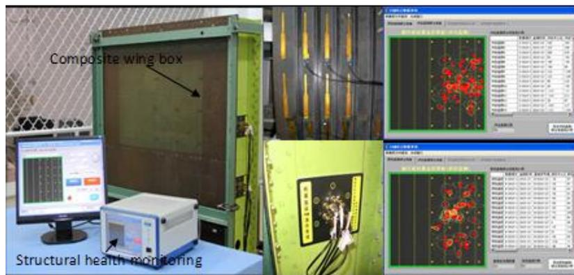
Figure 9. Demonstration system monitoring impact and delamination on the composite wing box.
