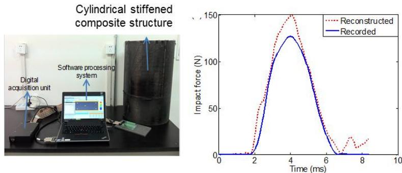
Figure 8. Photograph of impact monitoring system and reconstruction of impact force.
