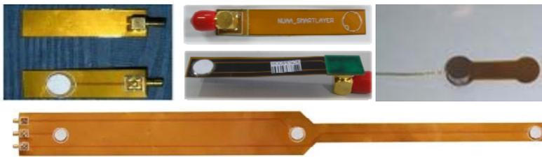
Figure 2. A series of PZT sensor layers with electromagnetic shielding.
