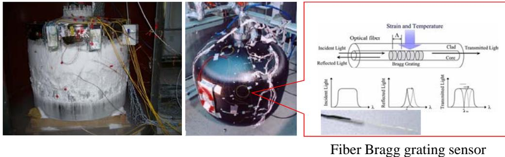
Figure 11. Strain and temperature monitoring using FBG sensors.
