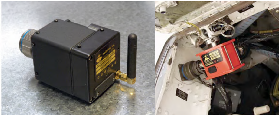
Figure 1. Wireless Flight Data Recorder (L) and Flight Data Recorder Installation on aircraft (R).
