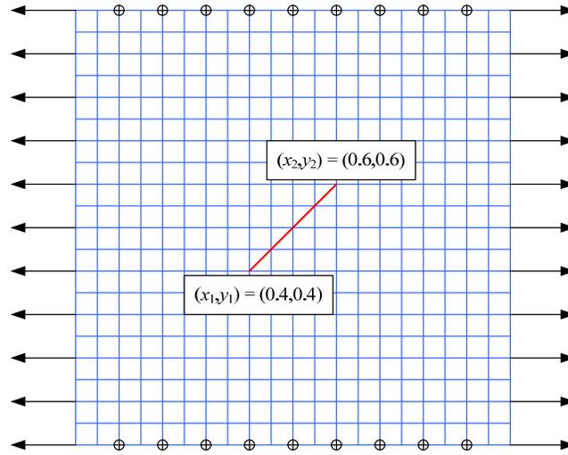
Figure 2. Mesh generation, crack orientation and sensor placement in numerical example.
