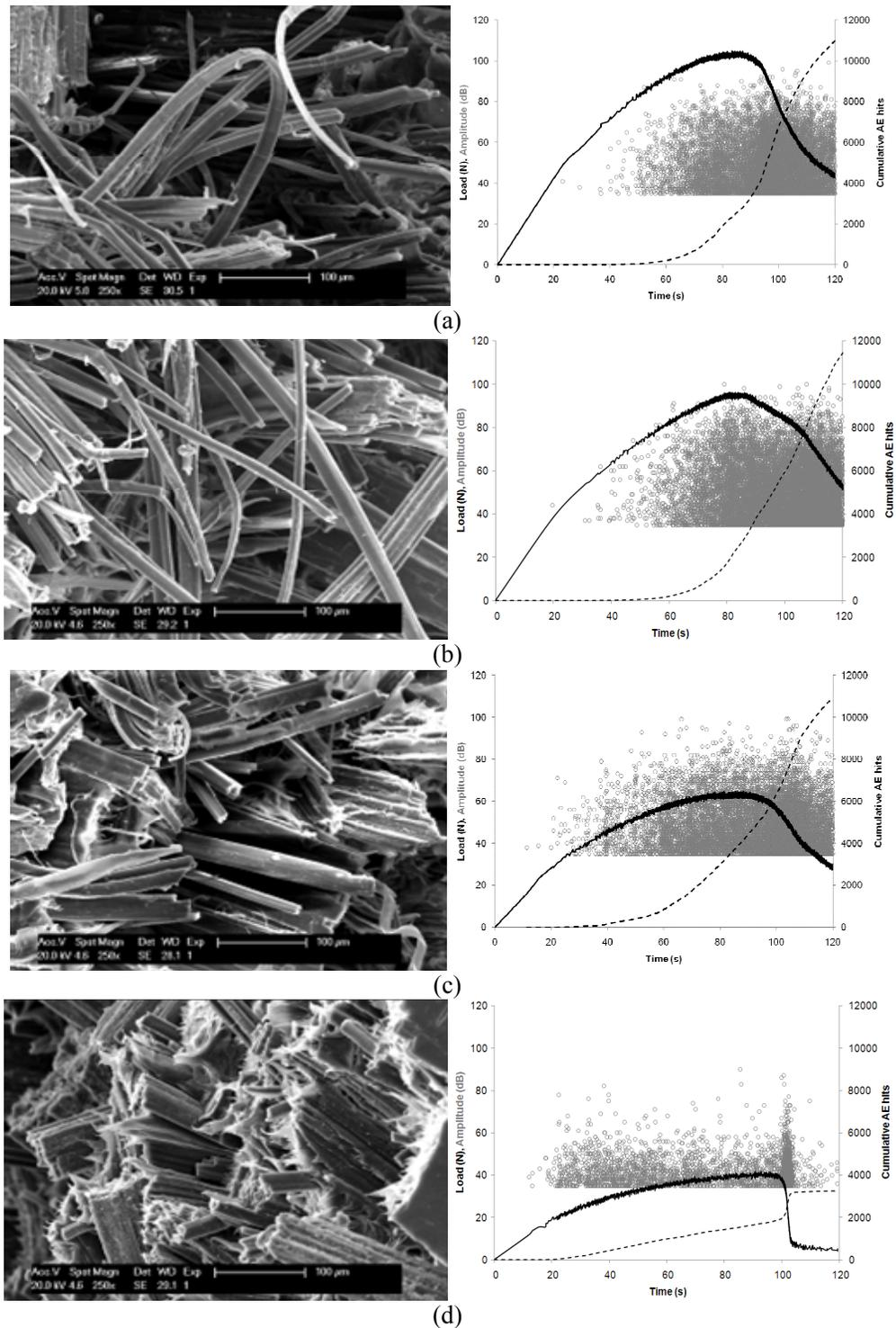
Figure 2. SEM fracture feature and EA analysis (Each individual event is indicated by a circle) during flexural test after three point bending test of hemp/PP composites, (a): as received, (b): Aged at 23°C 80%RH, (c): Aged at 70°C 80%RH, (d): Aged at 90°C 80%RH.
