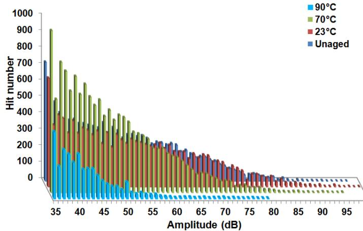
Figure 3. Acoustic emission amplitudes distributions for as received and aged NDF/PP composites.
