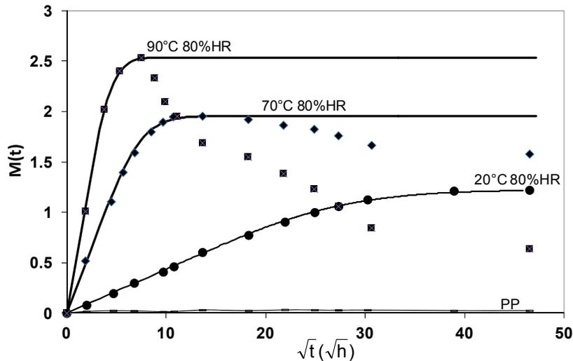
Figure 1. Water uptake variations as a function of the square root of time of the neat matrix and hemp/PP composites exposed to humid atmosphere (80% RH) at various temperatures. Solid lines are fits based on Fick's law.
