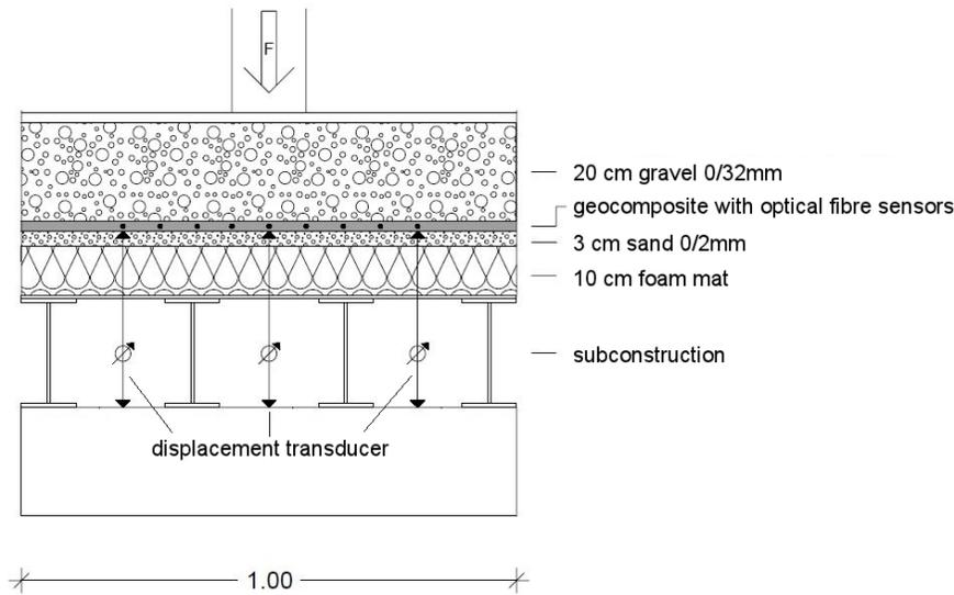
Figure 3. Cross-section of the test setup.
