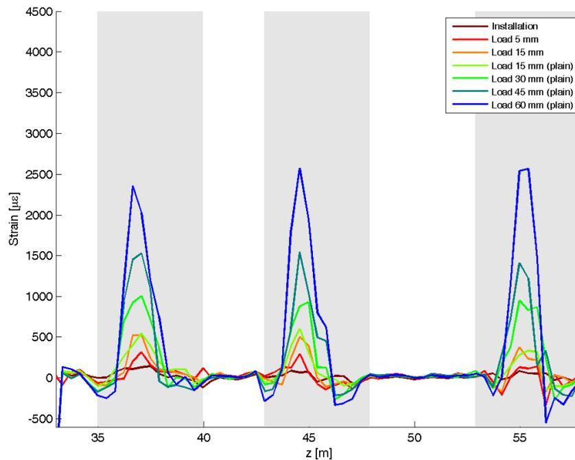
Figure 5. Results of distributed strain measurements, fiber samples 3, 4, 5 at the different deformation values induced by the hydraulic indenter load. The shaded areas correspond to the fiber sections that are integrated into the geosynthetic.
