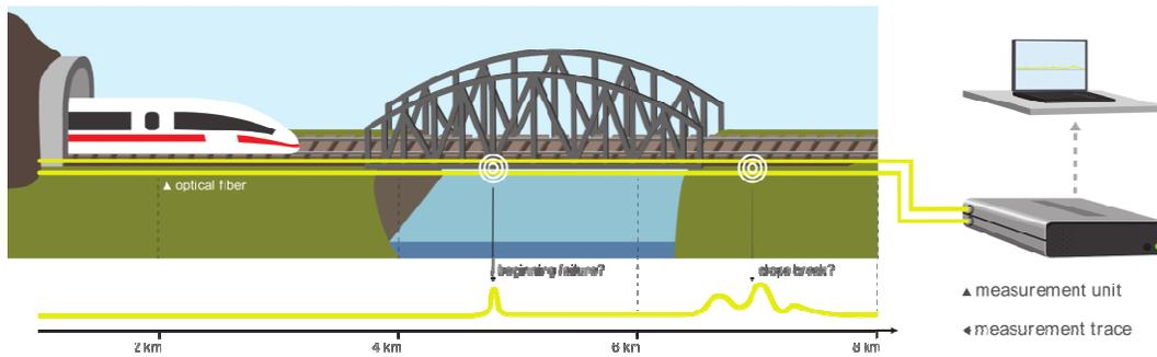
Figure 1. Distributed optical fiber sensors for deformation detection in large geotechnical structures.
