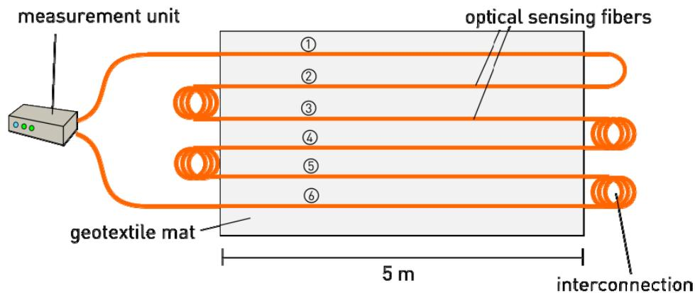
Figure 4. Layout of the optical fiber sensors embedded into the geosynthetic fabric at the settlement test bench.
