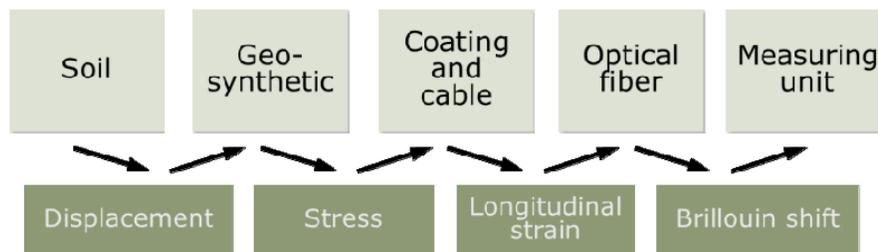
Figure 2. Transfer chain of the physical quantities from a displacement event in the soil to the measured sensor signal.
