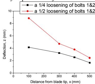
Figure 4. Variation in the amount of deflection upon half and quarter loosening of the bolt at different distances from the blade tip.
