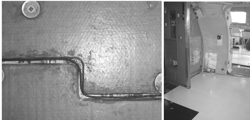
Figure 6. Part of the implementation area in a Boeing 737-500; left picture: the sensors (black wire) is placed between floor panels and right picture: partially re-sealed floor in the galley area with implemented sensor under the galley area and galley door.
