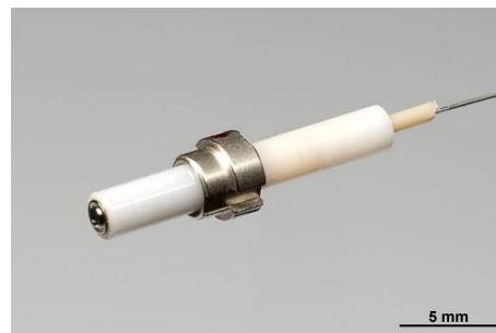
Figure 5. Modified DMI connector for embedding purposes.
