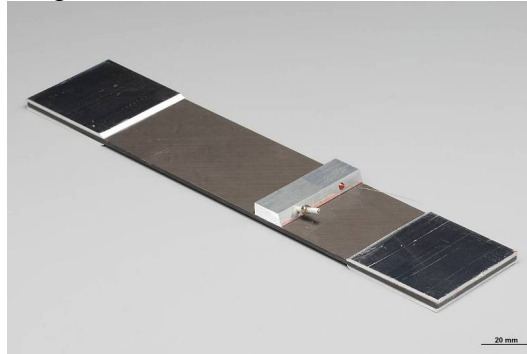
Figure 7. Specimen with prototype design embedded optical fibre connector assembly.
