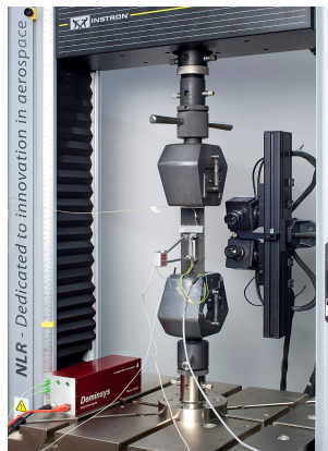
Figure 8. Test set-up with specimen in Instron 5882 static testing machine.
