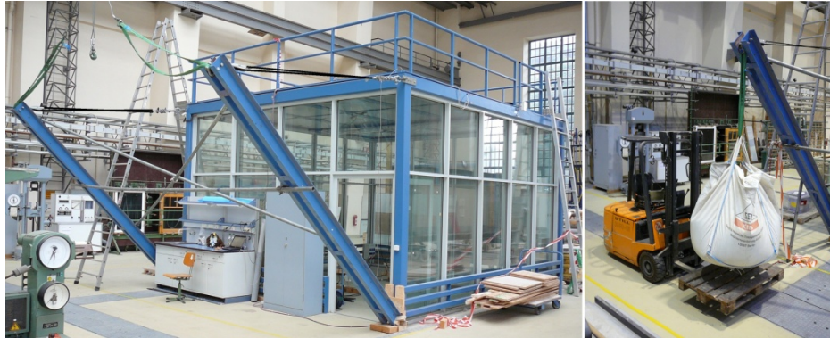
Figure 1. Test structure (left) and horizontal loading by a sandbag (right).
