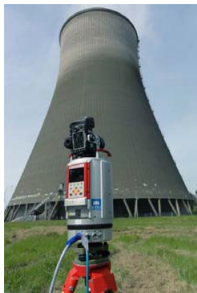
Figure 4. LIDAR in operation on a survey pillar.
