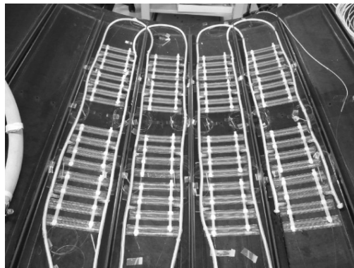
Figure 1. Hierarchical surface-crack monitoring system deployed on CFRP fuselage panel.
