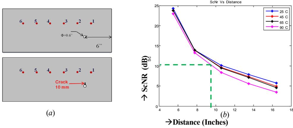
Figure 2. (a) Schematic of aluminum plate (with and without crack) attached with PZT elements, (b) and Scatter to Noise Ratio ( $ScNR_{aX}$ ) for different wave propagation distances under varying temperature conditions.
