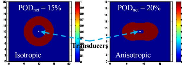
Figure 7. Comparison of single sensor coverage area for isotropic and anisotropic samples.
