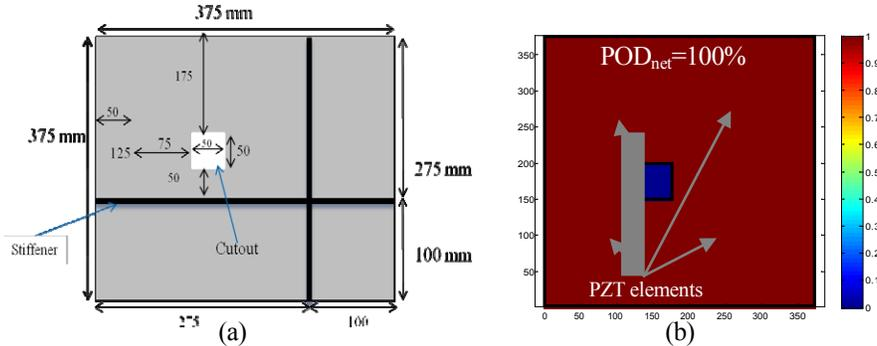
Figure 8. Demonstration of sensor network optimization tool (a) Schematic of aluminum structure with stiffeners and a cutout, and (b) Optimized sensor network.
