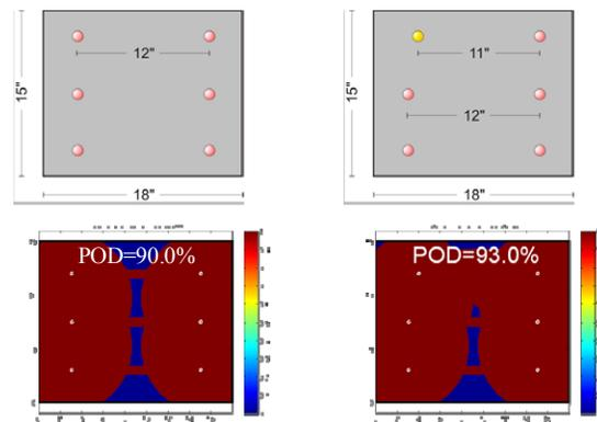
Figure 3. Effect of sensor placement on the  $POD_{net}$ .
