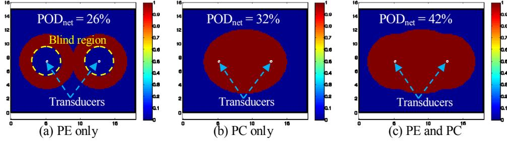
Figure 6. Comparison of coverage area with Pulse-echo and Pitch-Catch methods.
