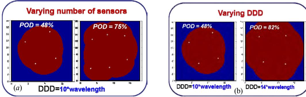
Figure 4. (a) Effect of number of sensors on  $POD_{net}$ , (b) Effect of varying DDD on  $POD_{net}$
