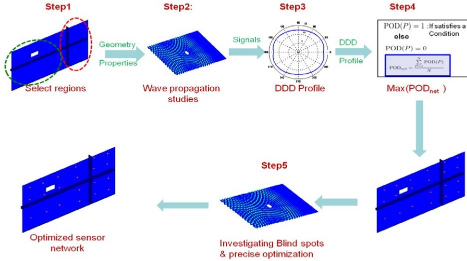
Figure 1. Schematic of the proposed approach for the sensor network optimization of SHM system.
