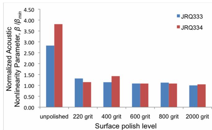
Figure 4. Dependence of acoustic nonlinearity parameter on surface polish level for two JRQ samples.
