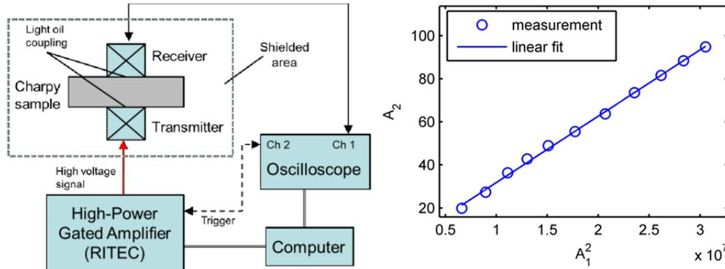
Figure 1. Laboratory schematic for nonlinear ultrasonic measurement (left), and representative measurement, showing linear growth of  $A_2$  compared to  $A_1^2$  (right). The slope of the linear fit is equal to  $\beta$ , the acoustic nonlinearity parameter.
