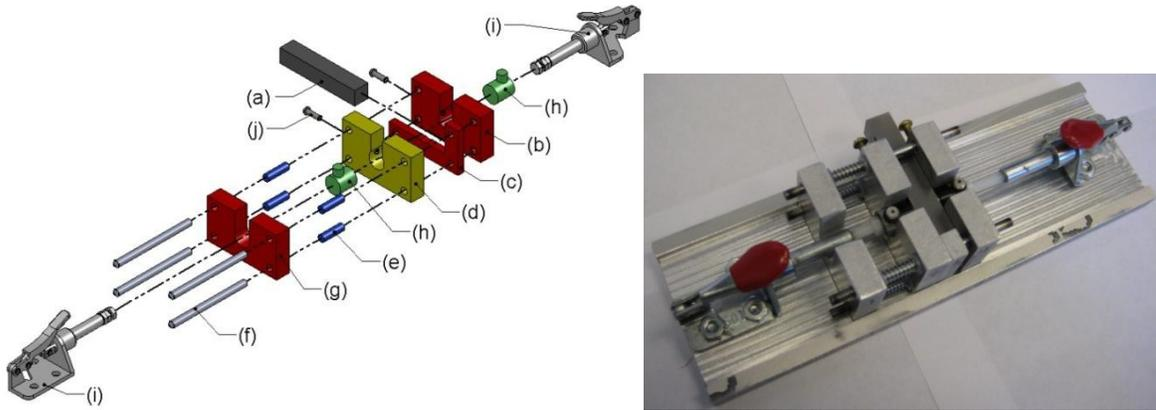
Figure 2. Exploded view of fixture design (left), and photograph of fixture with mounted sample and transducers. (right).
