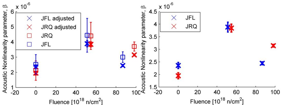
Figure 3. Acoustic nonlinearity parameter measured over fluence level for unadjusted results [1] and results adjusted to account for surface roughness effects (left), and adjusted results shown only for clarity (right).
