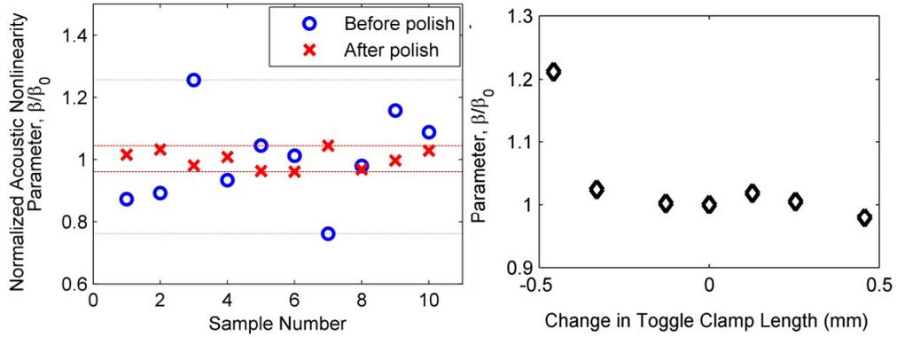
Figure 5. Normalized acoustic nonlinearity parameter before polish (polished to 600 grit) and after polish to 2000 grit (left). Variation in normalized acoustic nonlinearity parameter with change in toggle clamp length (right).
