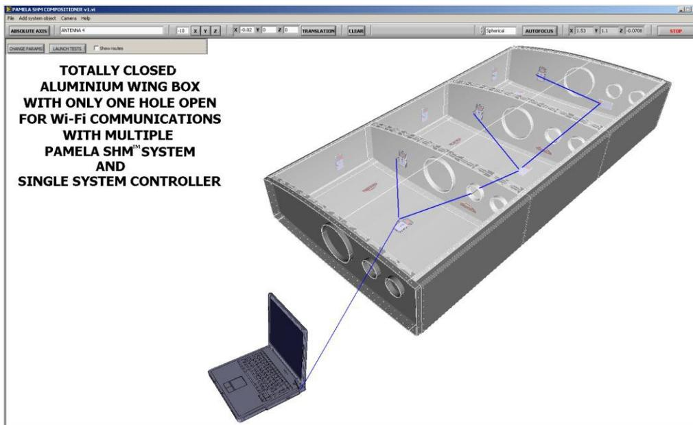
Figure 5. PAMELA SHM™ Composer HMI. Software tool for visualization of Wi-Fi communication paths in closed or open aerospace structure.
