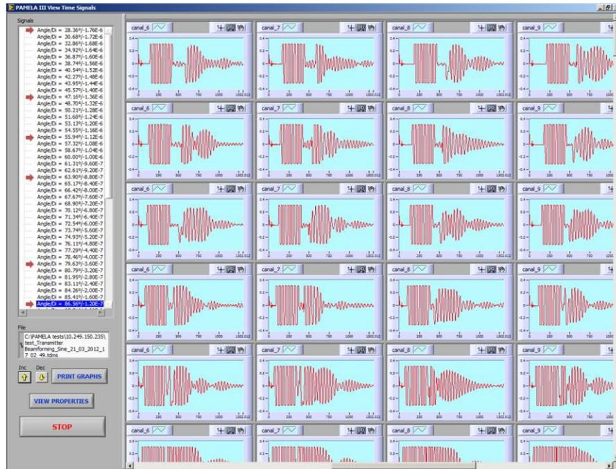
Figure 3. PAMELA SHM™ Visualizer HMI. Time signals obtained from a transmitter beamforming.
