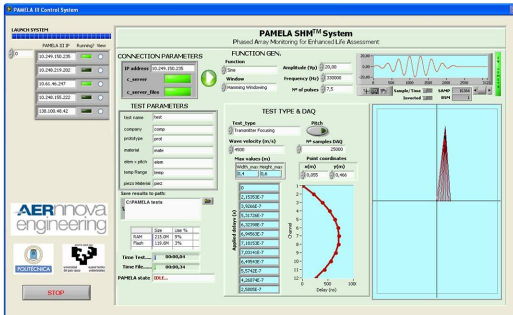
Figure 2b. PAMELA SHM™ System Controller HMI. Example of transmitter focusing test.
