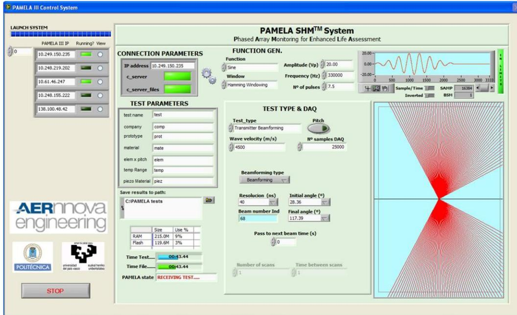
Figure 2a. PAMELA SHM™ System Controller HMI. Example of transmitter beamforming test.
