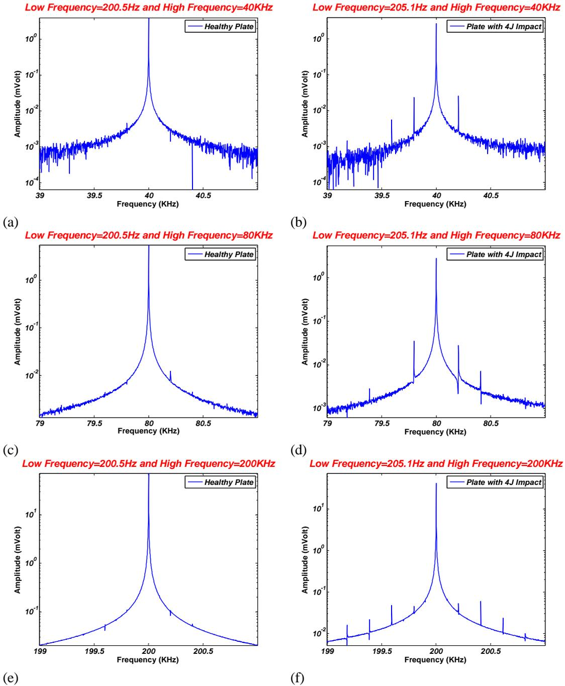
Figure 3. Spectral components of the sensor signal measured in a healthy (left) and a damaged (right) plate for various frequency values of ultrasonic carrier waves applied at the HFA. (a-b) 40KHz; (c-d) 80KHz; (e-f) 200 KHz. The damaged plate was subjected to 4J impact load.
