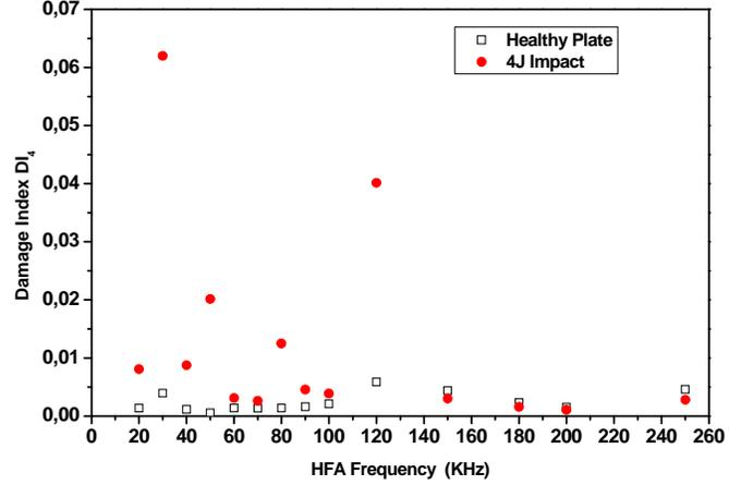
Figure 4. Variation of modulation factor  $DI_4$  as a function of the applied HFA actuation.
