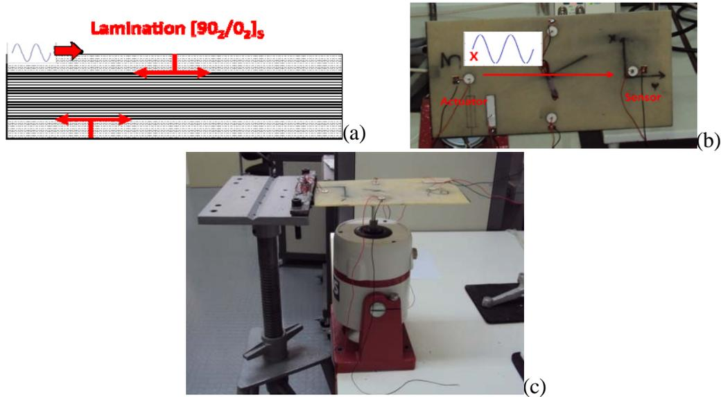
Figure 2. Experimental procedure (a) Possible generated damage in the composite plate due to impact vs wave propagation (b) Used pair of piezoceramics and (c) Cantilever experimental setup.
