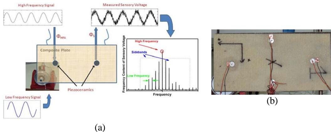
Figure 1. (a) Experimental setup and (b) Glass/Epoxy composite plate with two pairs of piezoceramic wafers attached.
