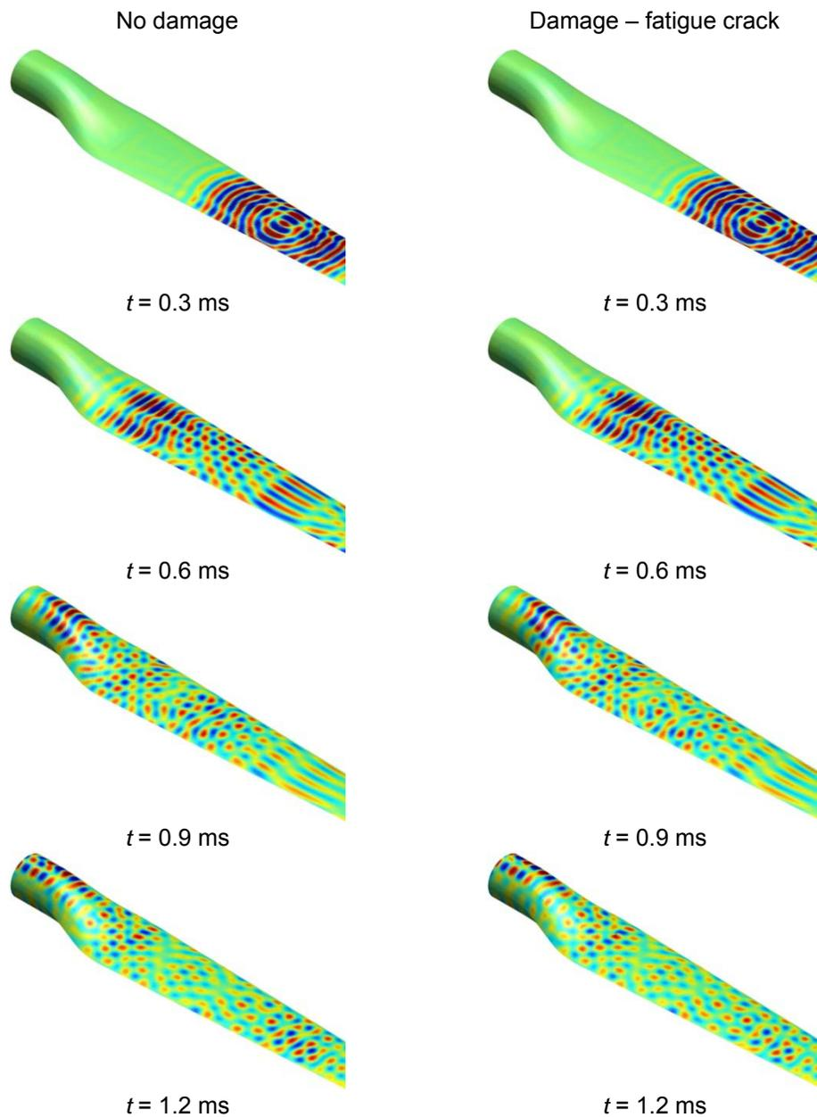
Figure 2. Wave propagation patterns obtained for a laminated composite wind turbine blade based on the transverse displacement component.
