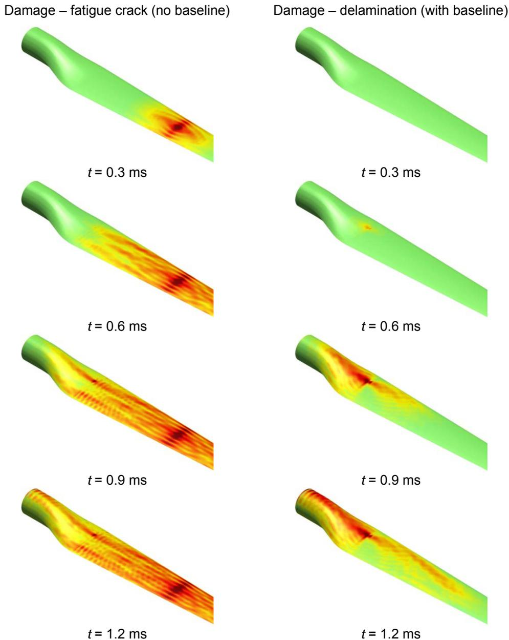
Figure 3. Evolution of RMS maps calculated for a laminated composite wind turbine blade based on the transverse displacement component.
