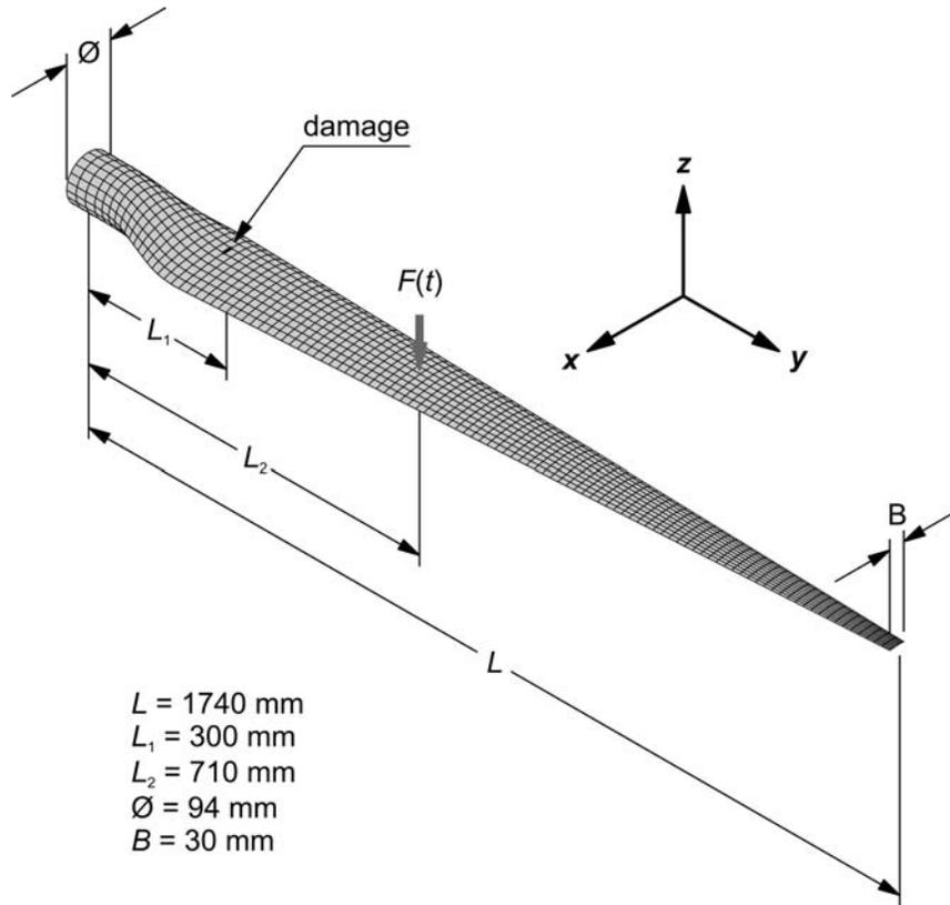
Figure 1. Geometry of a laminated composite wind turbine blade.
