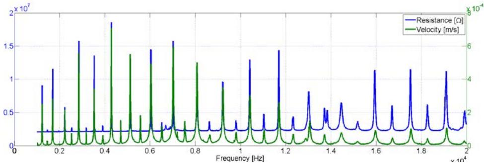
Figure 5. Comparison of mechanical and electrical spectra (sensor P12).
