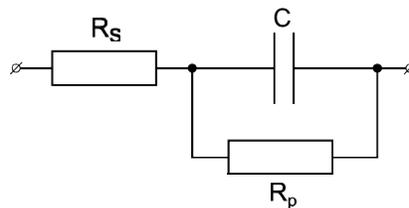
Figure 1. Equivalent circuit for a piezoelectric transducer.
