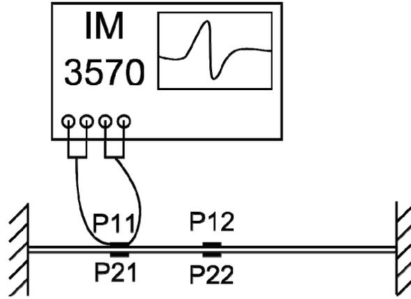
Figure 2. Experiment setup for impedance investigation.
