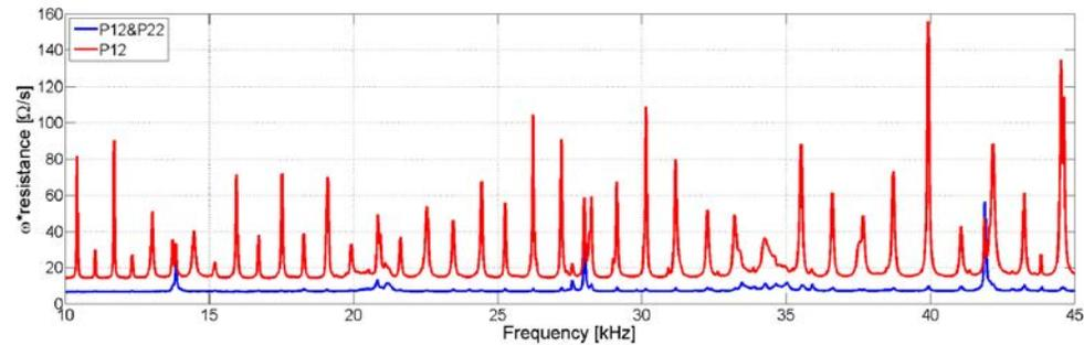
Figure 7. Comparison of transducers connected in antiphase spectra and a simple sensor.
