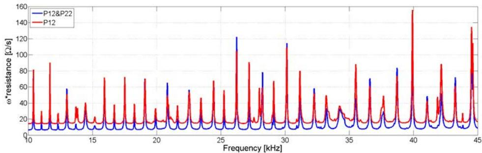
Figure 6. Comparison of transducers connected in phase spectra and a simple sensor.
