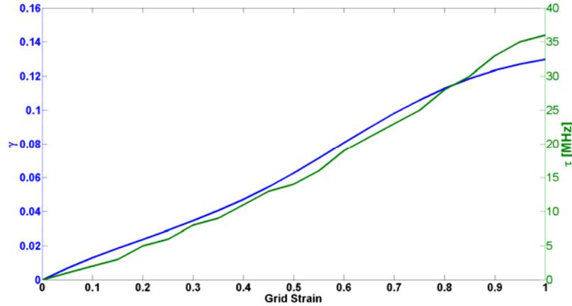
Figure 3. Frequency shift and normalized scale factor versus grid strain, for the central antennas of a grid of 5 dipoles.
