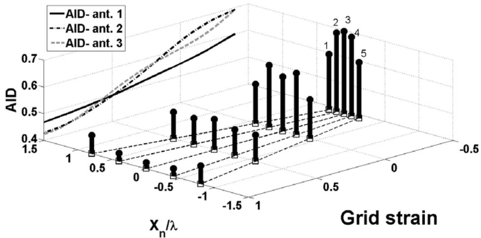
Figure 2. Histogram representation of the grid analog identifier profile at a given frequency versus overall grid strain and position of the sensor over the surface, for a grid of 5 dipoles.
