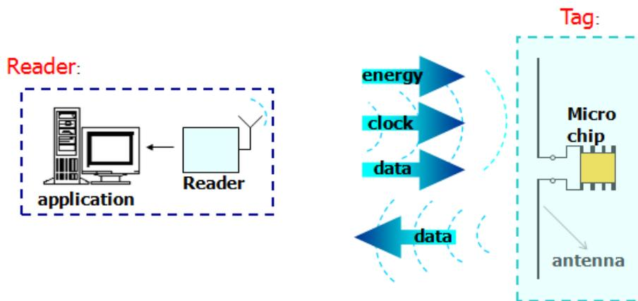
Figure 1. scheme of an RFID system, comprising the reader and the tag(s).
