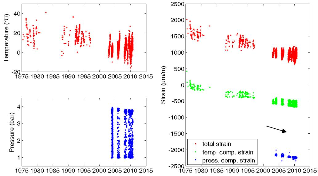
Figure 7: Strain measured on elastic zone.
