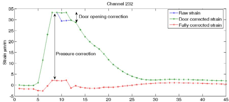
Figure 5. 24-hour test: rising pressure, opening door, stopping compressor, opening gate. Example of sensor strain compensation.
