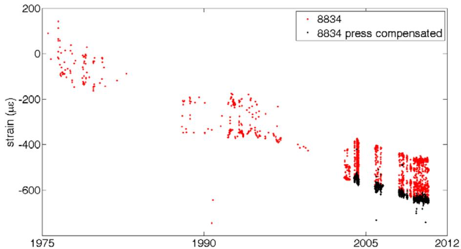
Figure 6. Pressure compensated strain.
