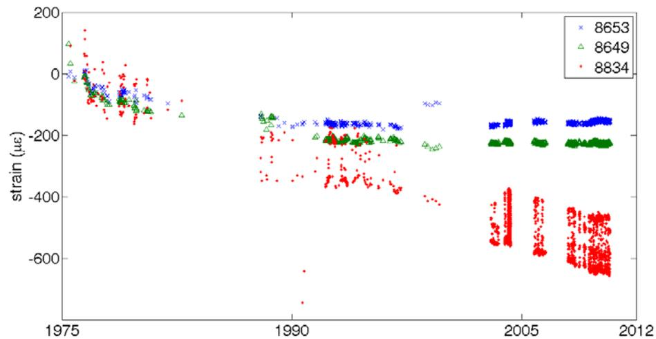
Figure 4. 35-year strain measurement performed by 3 different sensors.
