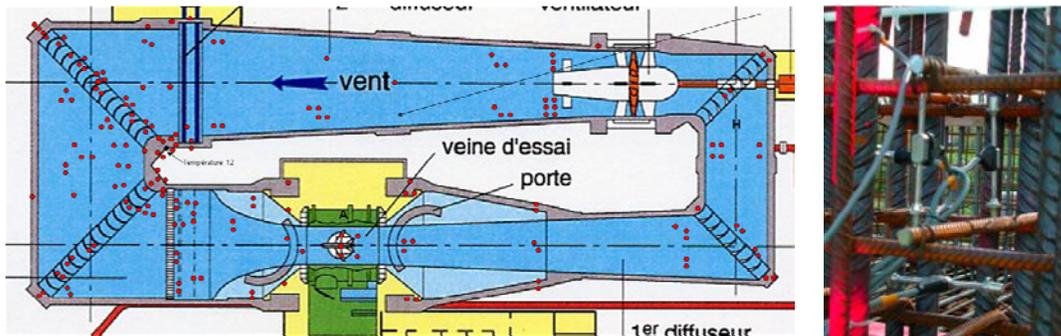
Figure 3. (left) Wind Tunnel instrumentation: red dots represent VW extensometers. (right) View of VW extensometers before concrete pouring (2).
