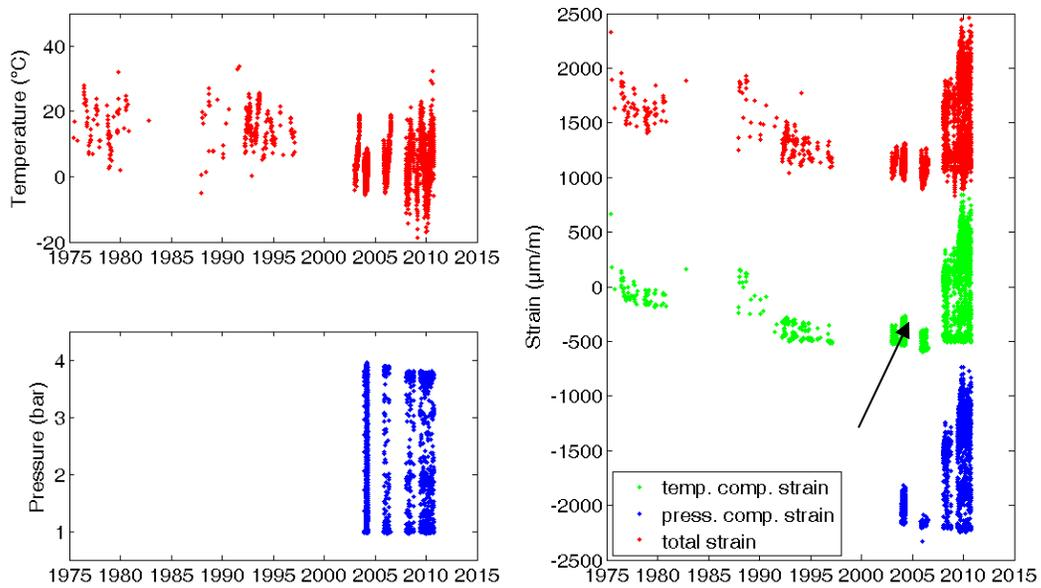
Figure 8. Strain measured on cracked zone.
