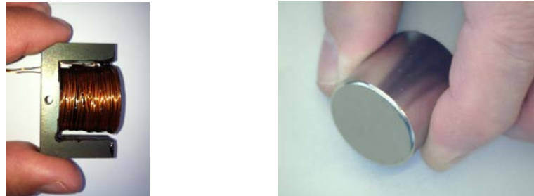
Figure 2. Components for spin energy harvester: Coil and laminated transformer core (at left), neodymium iron boron magnet (right).
