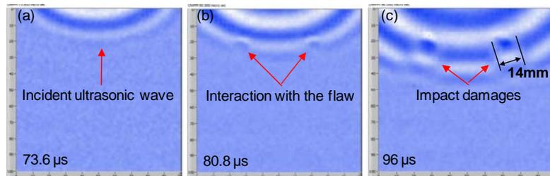
Figure 5. Freeze frames of UWPM showing incident ultrasonic waves and its interaction with the flaw (a) at 73.6  $\mu$ s (b) at 80.8  $\mu$ s, incident waves interact with the impact damage (c) at 96  $\mu$ s, scattered waves indicate impact damage detection.
