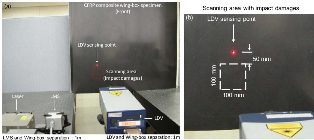
Figure 3. (a) Experimental setup for impact damage evaluation in carbon fiber reinforced plastic composite wing box specimen using hybrid laser ultrasonic generation/LDV sensing and (b) Scanning area in the target specimen with LDV sensing point.
