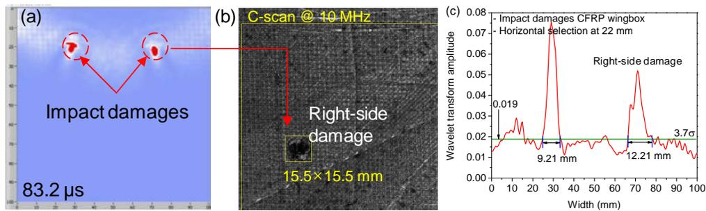
Figure 4. Impact damages in the carbon fiber reinforced plastic composite wing box detected (a) on wavelet transformed ultrasonic propagation movie result and (b) Damage size comparison with the C-scan result (c) Further analysis of the result for damage size estimation.
