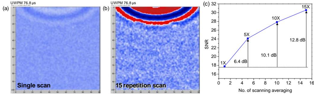
Figure 2. UWPM freeze frames comparison at same time frame and color scale showing improvement in signal intensity due to repeat scanning technique. (a) Single scan (b) 15 repeat scanning. (c) Improvement in SNR for different number of repeat scans.
