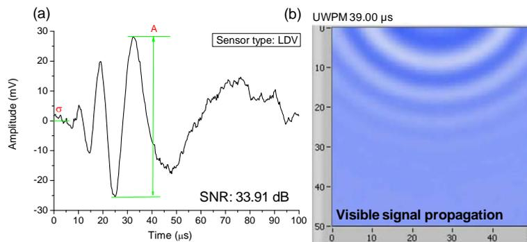
Figure 1. (a) Time domain ultrasonic signal with respect to one impinging point, and (b) visible ultrasonic wave propagation movie (UWPM).
