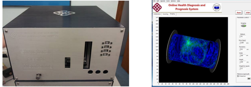
Figure 6. The online diagnosis system (left: integrated system; right: UFI).
