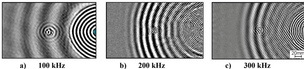
Figure 3. Reflection and mode conversion from  $S_0$  at a 50% flat bottom hole of 20 mm diameter in a CFRP plate according to Tab. 1.
