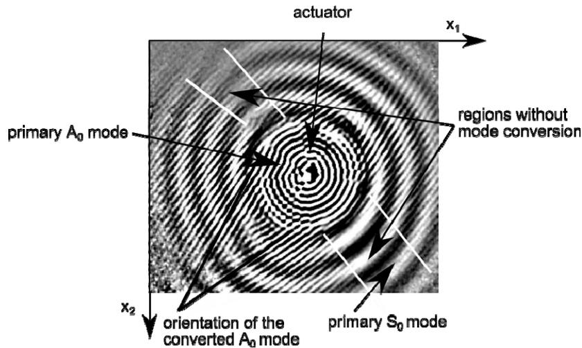
Figure 5. Lamb wave propagation in a CFRP plate at 200 kHz, excited by an actuator in the center (displayed area 300 mm x 250 mm).
