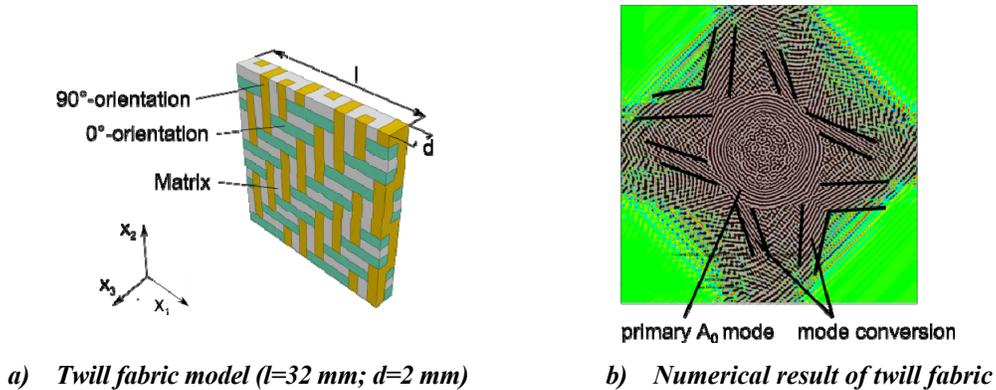
Figure 8. Numerical model and solution of a twill fabric plate at 250 kHz.
