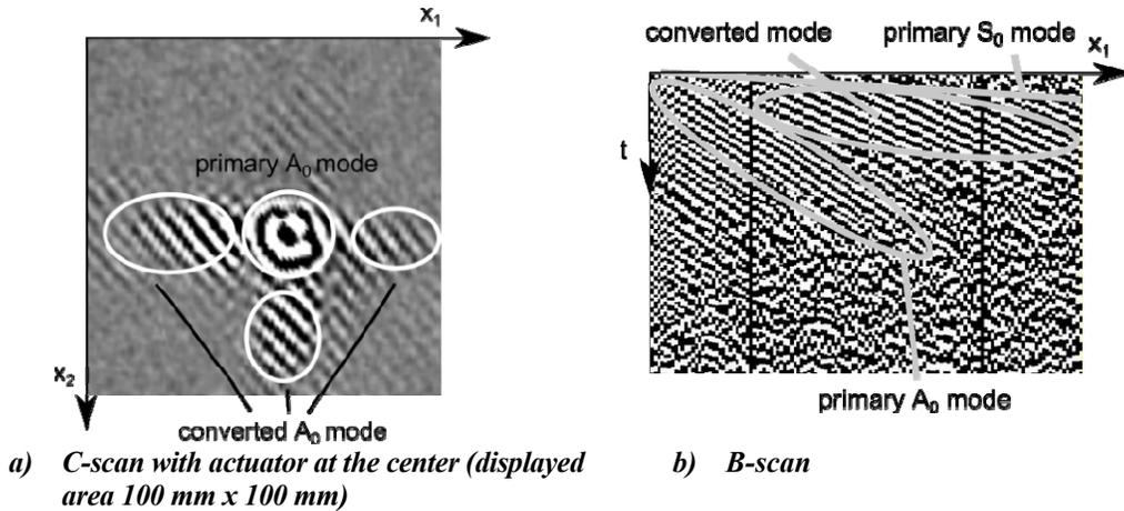
Figure 7. Experimental results for a single layer twill fabric plate at 50 kHz.
