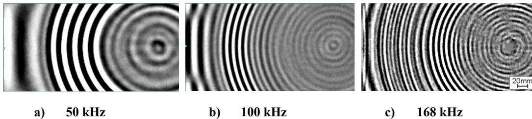
Figure 2.  $S_0$  edge reflection in a PMMA plate without mode conversion.
