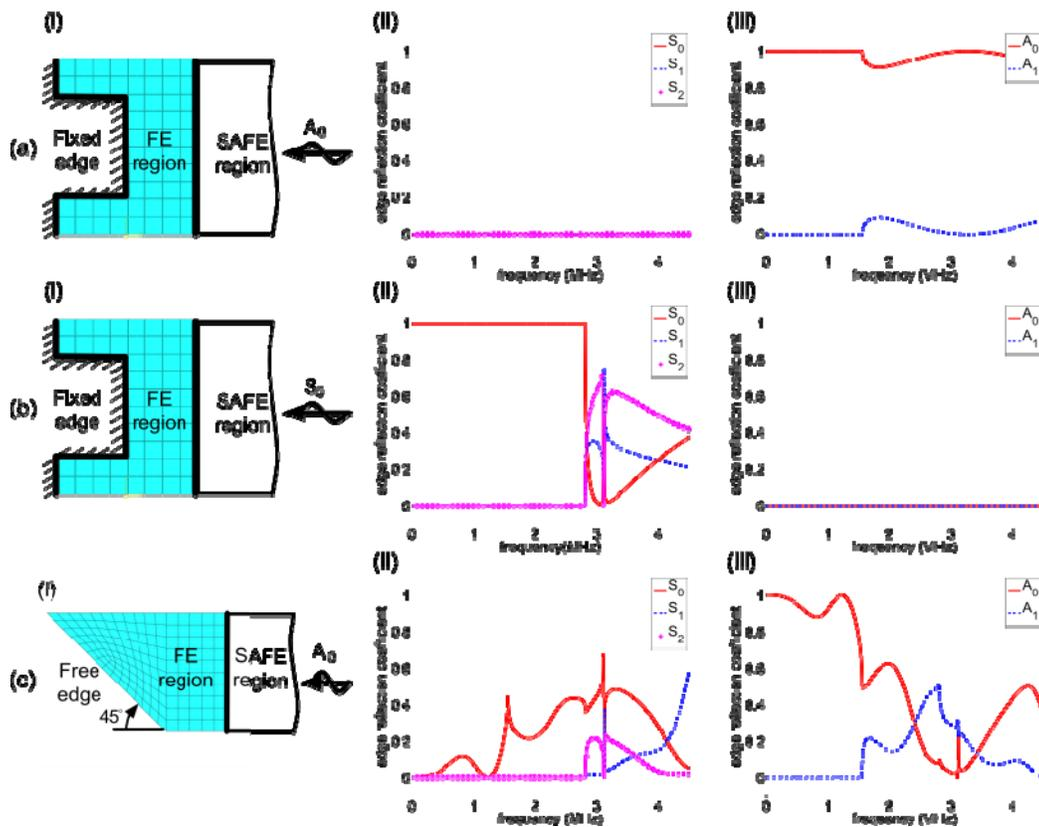
Figure 4. (a)  $A_0$  mode reflection by a fixed symmetric end plate: i) SAFE-FE model, ii) symmetric mode reflection, and iii) anti-symmetric mode reflection; (b)  $S_0$  mode reflection by a fixed symmetric end plate: i) SAFE-FE model, ii) symmetric mode reflection, and iii) anti-symmetric mode reflection; (c)  $A_0$  mode reflection by an inclined free edge ( $45^\circ$ ): i) SAFE-FE model, ii) symmetric mode reflection, and iii) anti-symmetric mode reflection.
