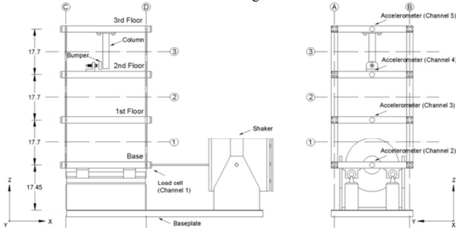
Figure 1. Mechanical drawing of the three-storey frame structure.
