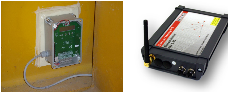
Figure 2. The “Smartbrick” WASHM platform installed on a structure (left) and wireless sensor node “Smartmote WS ” to build up a wireless sensor network on a structure (right).
