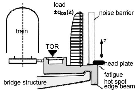
Figure 1. Cross-section of a bridge with noise barrier and the detail of the fatigue hot spot.
