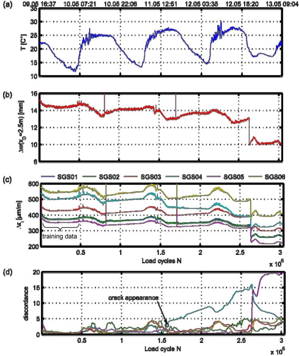
Figure 5. Compressed data of specimen T05. (a) temperature, (b) deflection range  $\Delta f = f_{max} - f_{min}$  measured by the deflection transducer, (c) strain range of SGS01 to SGS 06 and (d) outlier of the extracted feature.
