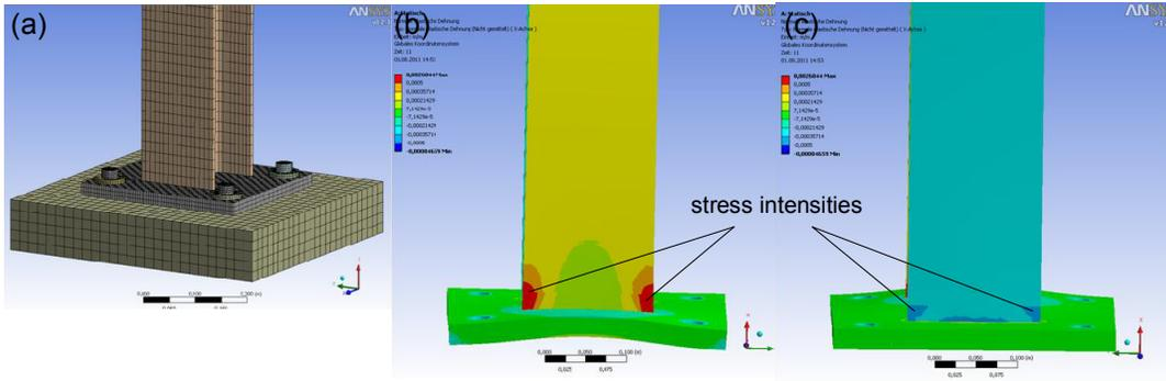
Figure 3. Finite element model to determine stress intensities. (a) discretization, strain in x-direction (deflection in y-direction) (b) tensioned flange and (c) compressed flange.
