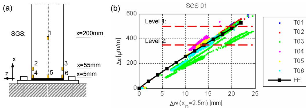
Figure 4. Comparison of FE results with the measurements. (a) Detail of the strain gauge sensor distribution and (b) strain in x-direction of SGS 01 according to the deflection of the beam.
