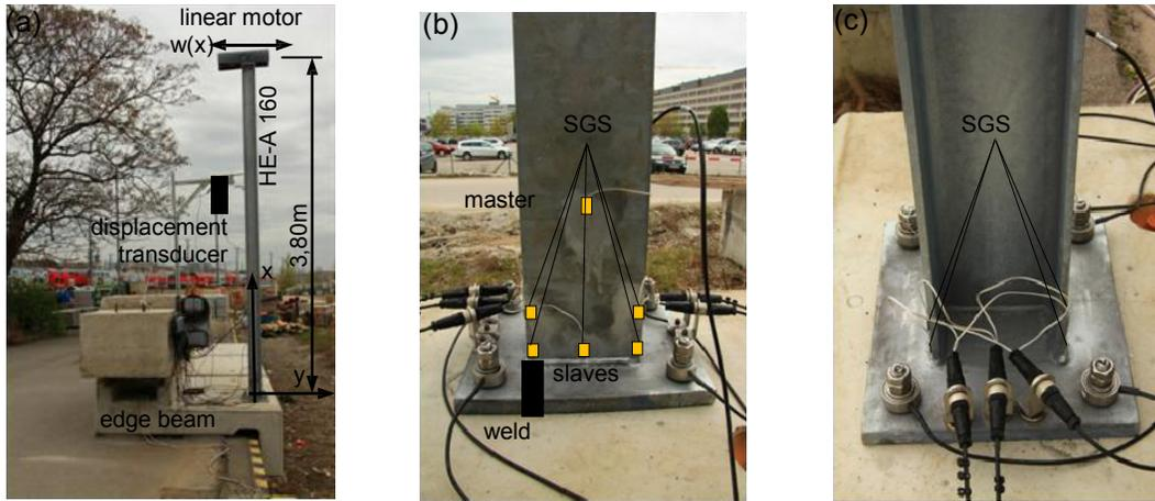
Figure 2. Experimental setup. (a) Noise barrier pillar on edge beam with electrodynamic vibration exciter on top, (b) strain gauge sensor (SGS) distribution and (c) coupling of tensioned and compressed sensor.
