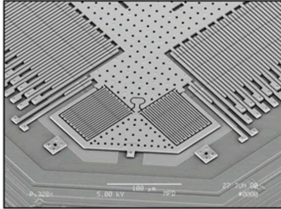
Figure 2: A commercial accelerometer, seen by SEM. The seismic mass is made by a thin film of polycrystalline silicon. The displacement is measured using differential capacities realized by inter-digital electrodes. Figure by Analog Devices ([www.analog.com](http://www.analog.com)).
