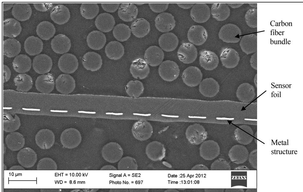
Figure 4: SEM picture of a thin sensor for the measurement of local dielectric function embedded in a carbon fiber compound (CFRP). The carbon fiber bundles have diameters of about 8  $\mu\text{m}$ . The sensor foil is 10  $\mu\text{m}$  thick. Within the sensor foil the metal structures appear as a broken white line.
