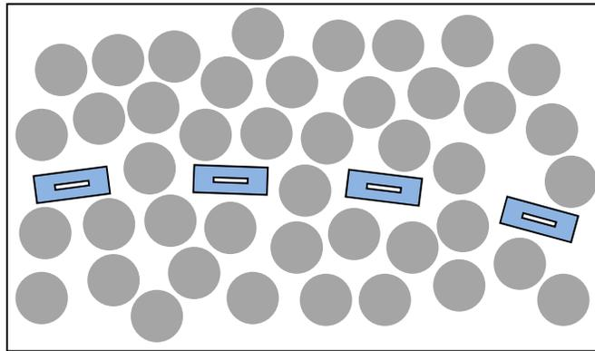
*Figure 5: Idea of a future sensor for the dielectric function of the CFRP. The sensor is reduced to a net of single fibers which adapt to the carbon fiber structure. This sensor net permits a minimum impact of the sensor to the structure.*
