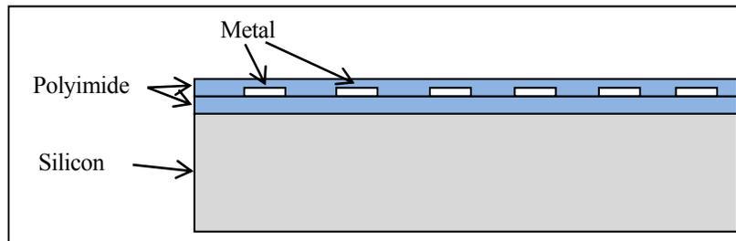
Figure 3: A dielectric sensor made by use of polyimide technology. A polyimide film is prepared on a silicon wafer. Next, the metal is deposited and structured. Additionally, a second polyimide layer is deposited and structured. Finally, the polymer – metal – polymer sandwich is removed from the silicon substrate.
