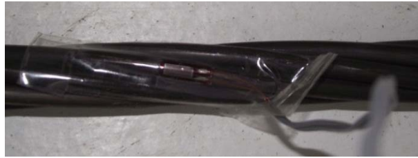
Figure 4. Placement of strain gages.
