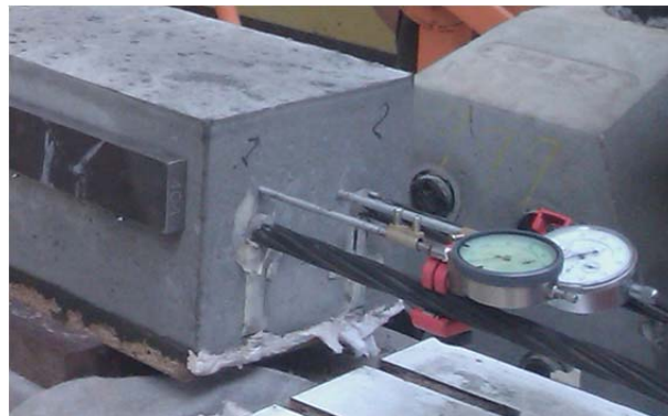
Figure 6. Placement of the transducer displacement for measuring penetration \delta .
