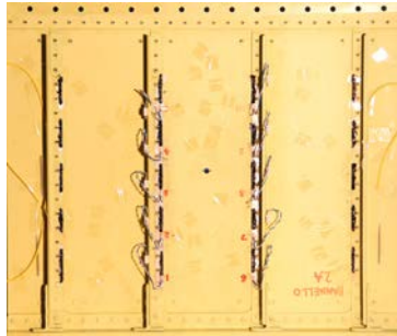
Figure 1. Typical aeronautical panel consisting in a skin stiffened through some riveted stringers. 20 FBG sensors have been applied to monitor crack propagation.
