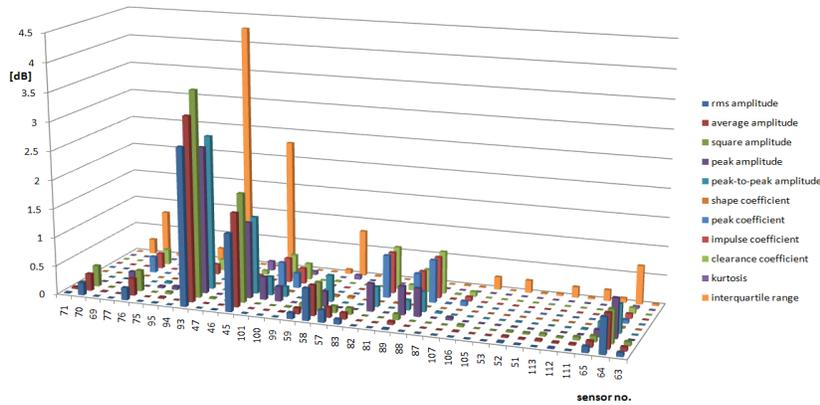
Figure 1. Selected measures relative values due to secondary damper fault.
