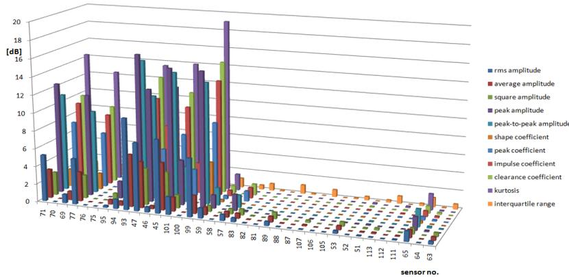
Figure 2. Selected measures relative values due to primary spring fault.
