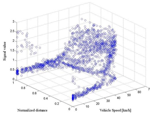
Figure 3. RMS values of vibration signal in the Z direction with regard to speed and the normalized distance from the initial position of the vehicle.
