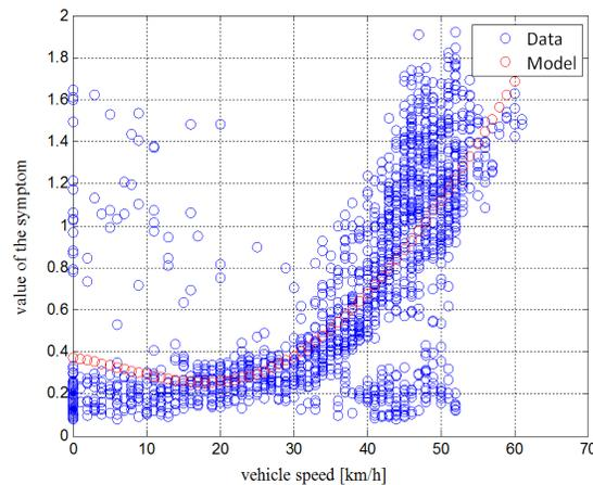
Figure 7. The proposed model fitted to the RMS acceleration value for all tramway passages on a given track section.
