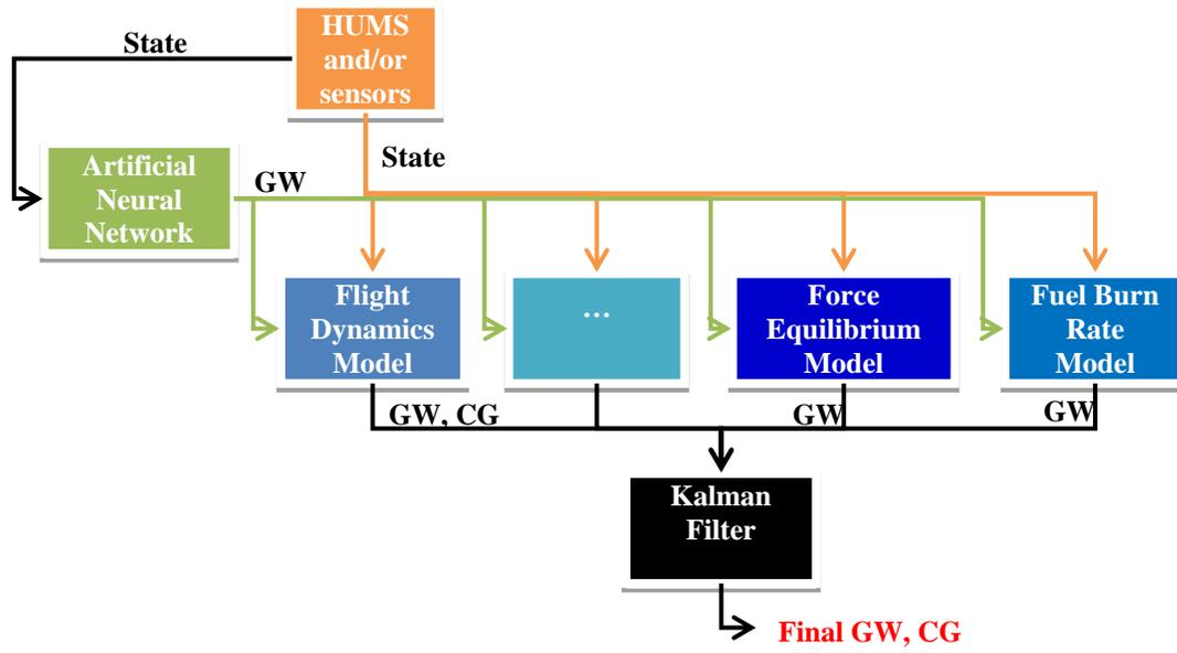
Figure 6. Multiple sources of GW and CG data combined with a KF and NN.
