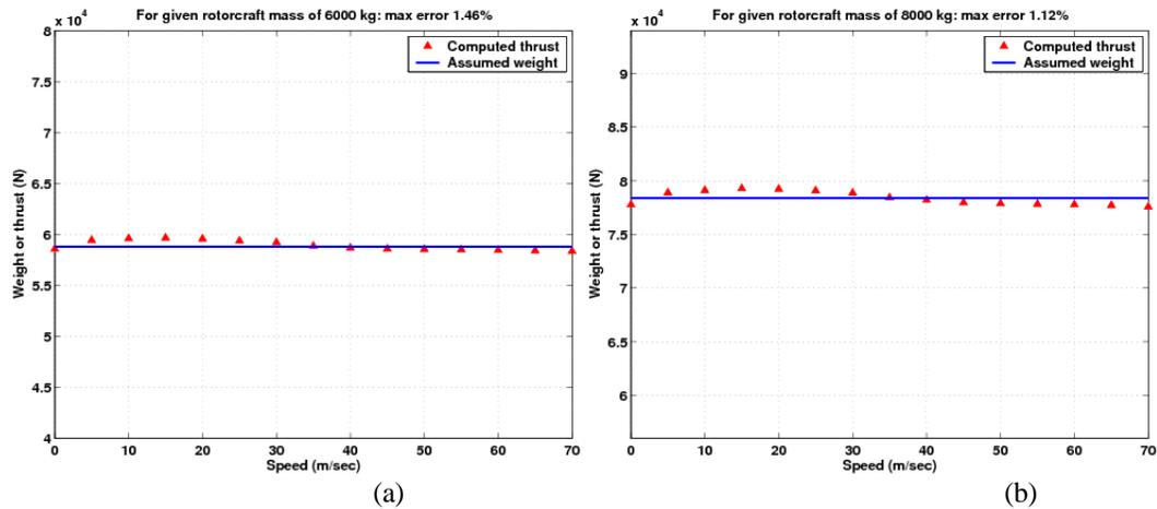
Figure 2. Comparison of computed thrust and given weight values for various speeds: (a) for a given rotorcraft mass of 6000 kg (the maximum percentage error is 1.46%); (b) for a given rotorcraft mass of 8000 kg (the maximum percentage error is 1.12%).
