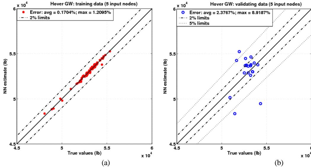
Figure 4. True values vs. predicted values: (a) training set (the average error is below 0.2%); (b) validating set (the average error is below 2.5%). Among 98 total data points, 78 were used for training and 20 for validating.
