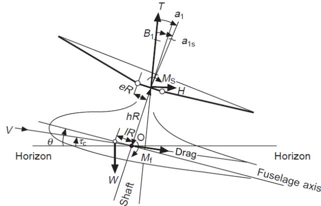
Figure 1. Longitudinal forces and moments of a generic helicopter [6].
