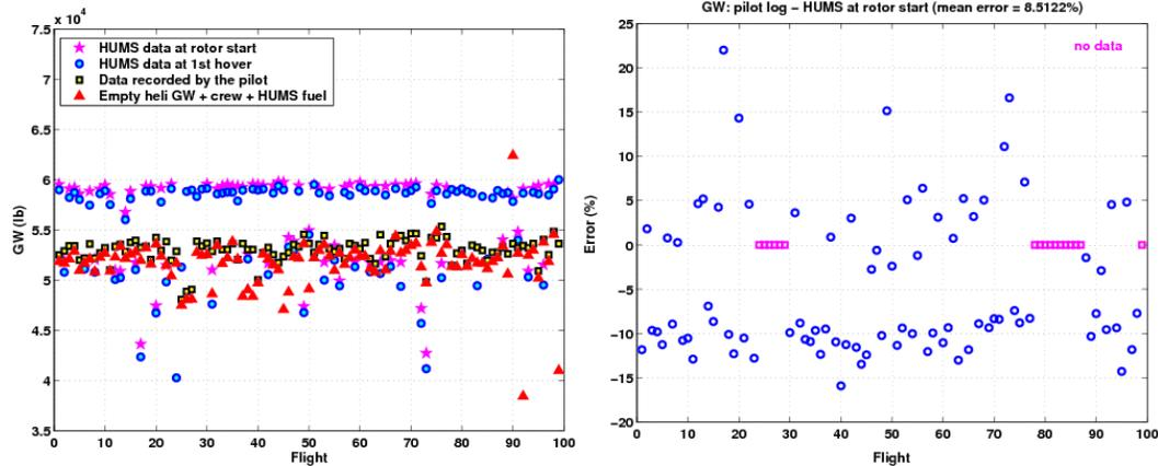
Figure 3. (a) Aircraft Gross Weight (lb) provided by: (1) HUMS at rotor start, (2) HUMS at first hover, (3) pilot at the beginning of the flight, (4) sum of empty weight, crew (from pilot's log) and fuel from HUMS; (b) Absolute error the average error is 8.5%.
