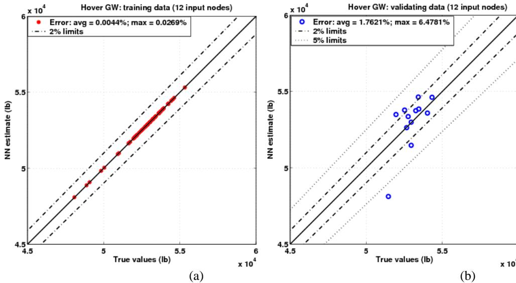
Figure 5. True values vs. predicted values: (a) training set (the average error is around 0.004%); (b) validating set (the average error is around 1.8%).
