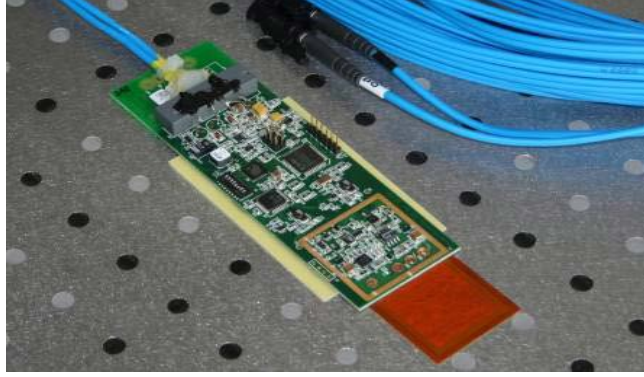
Figure 5 Complete realization of a sensor node with PZT sensor (red) and a duplex optical fiber cable for optical power supply and communication (blue)
