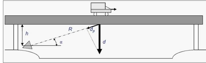
*Figure 5. Example for the geometry of a measurement of a bridge and the single components of the displacement [RICCI 2009].*
