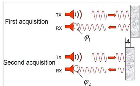
*Figure 4. Principle of the interferometric determination of object changes [RICCI 2009].*
