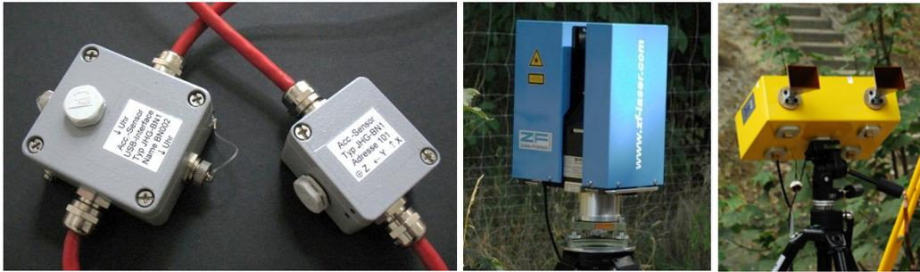
Figure 2. Low-cost accelerometer sensor system (left), TLS (middle) and IBIS-S (right).
