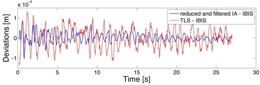
Figure 10. Deviations of displacements in comparison to IBIS-S.
