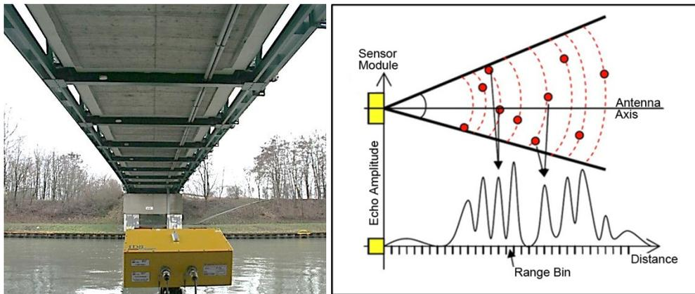
*Figure 3. Example of a structure with “natural” corner reflectors (left) [RIEDEL and LEHMANN 2012] and principle of signal detection (right) [RICCI 2009].*
