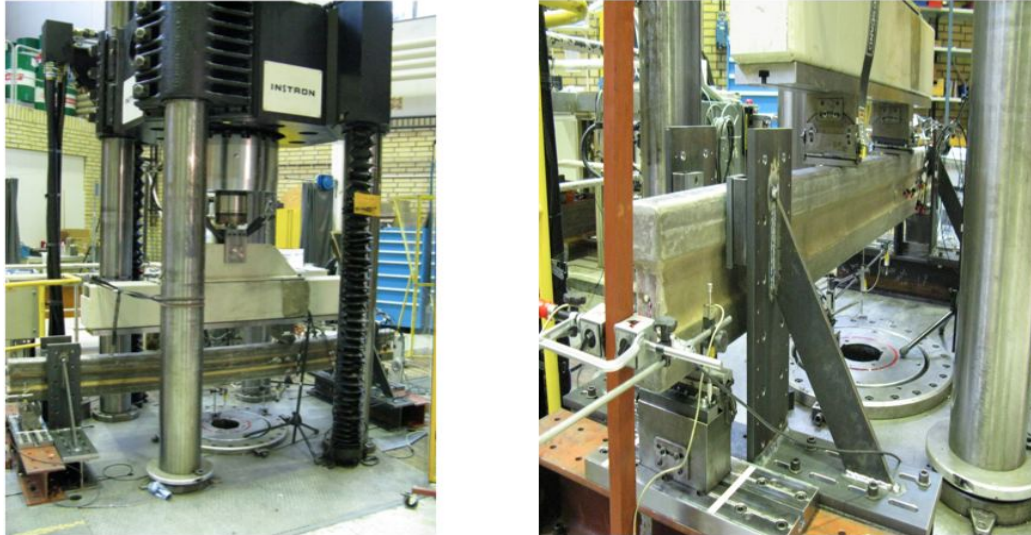
Figure 2. Left: The Instron machine. Right: The test beam ready for the start of the test.
