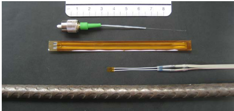
Figure 4. Relative dimensions of reinforcement steel, glass fiber and strain gauge.
