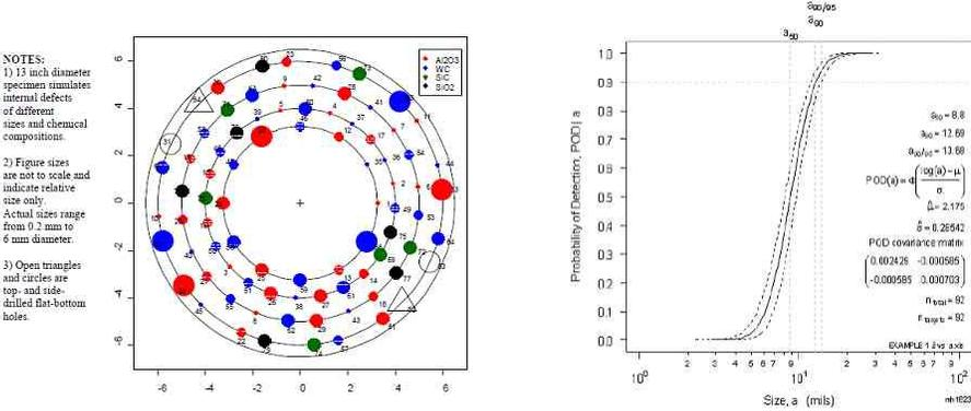
(a) UT internal target specimen (b) Example of PoD(a) curve
