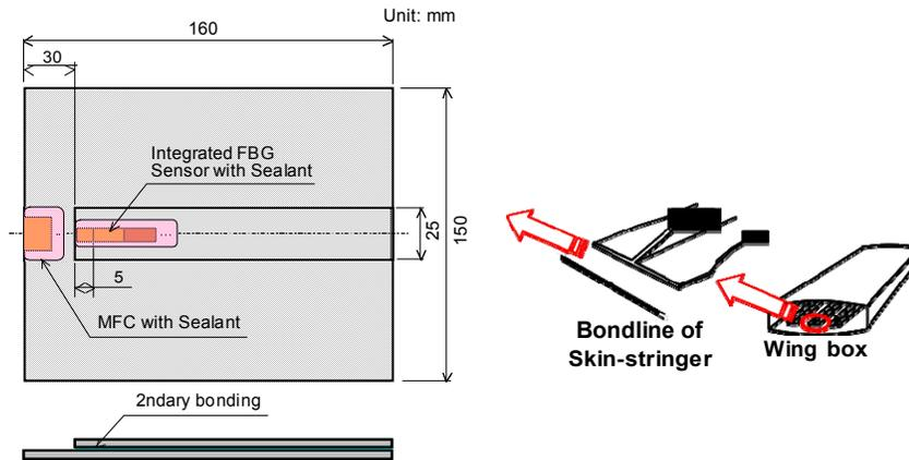
Figure 4. Schema of a fundamental coupon specimen.
