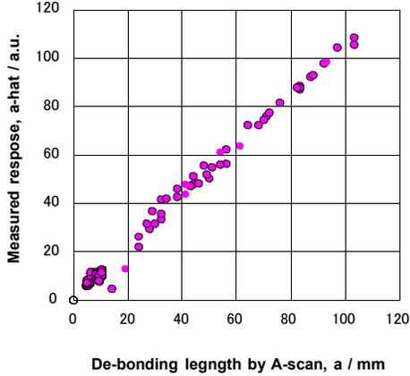
Figure 6. relationships between measured response by SHM and de-bonding length by A-scan.
