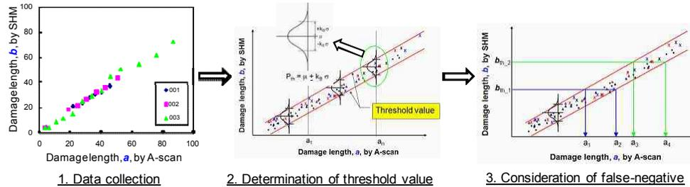
Figure 3. Outline of determination of threshold values and actual debonding length.
