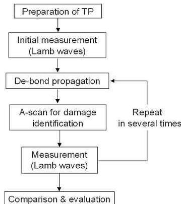
Figure 5. Test sequence in one specimen.
