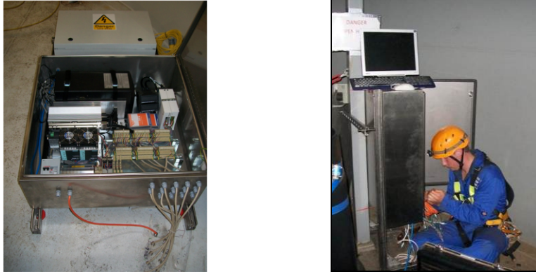
Figure 3. Data Acquisition Unit (left) and Commissioning System (right).
