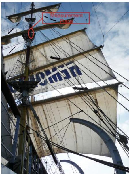
*Figure 2. Foremast of STS Dar Młodzieży with marked FBG sensors location.*
